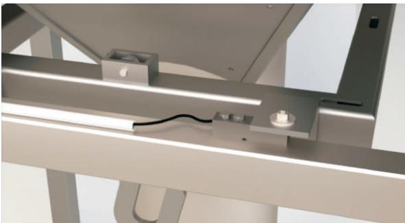
**SCALE** for commercial weighing while filling the bag. Needs to be calibrated after transportation of more than 200 km.
